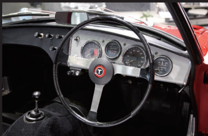
The instrument panel mirrors the same curves as the hood. In later models, the aluminum panel around the gauges was changed to black.
