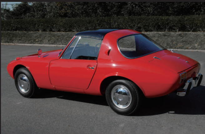
The roof panel was secured with six bolts, allowing for easy removal and a quick transition to open-top driving.
