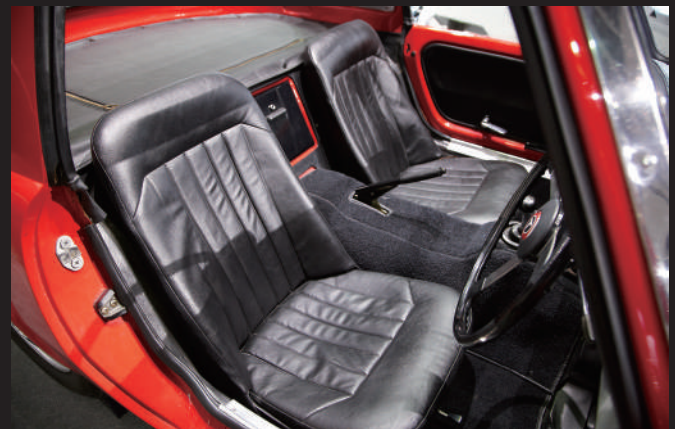
Both the driver and passenger seats could only slide forward and backward. A thick side member ran between the seats to maintain the body's rigidity.
