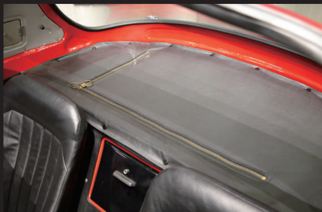
You can unzip the section behind the seat to store the roof. The roof, hood, and trunk lid are made of lightweight aluminum.
